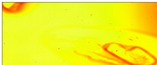
Picture 11. t.p on 142.9 °C, end crystal melting acetylsalicylic acid
