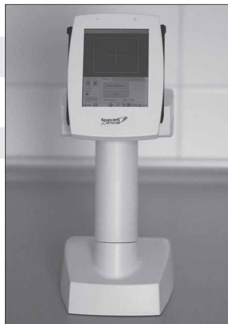
Figure 2. The Spectroshade - dental spectrophotometer
